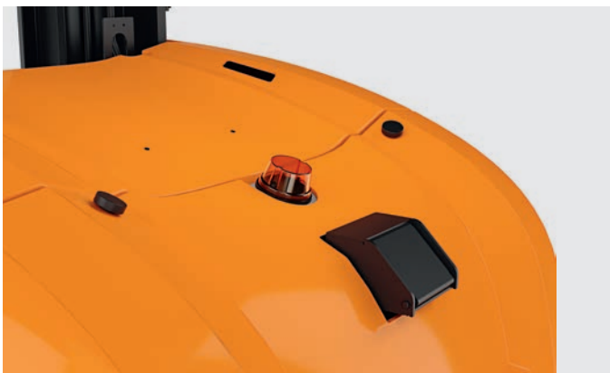
Fast charging for optimum availability: direct charging access on the PXV is key and makes handling the charging connector a lot easier for all operators
