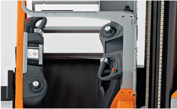
Maximum safety and flexibility when operating the truck thanks to display and control elements that can be positioned on the load end or mast side to suit requirements
