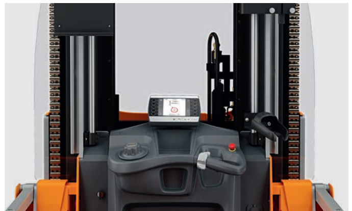
Safety and efficiency with everything in view: the mast ensures a clear view in the drive direction at all times
