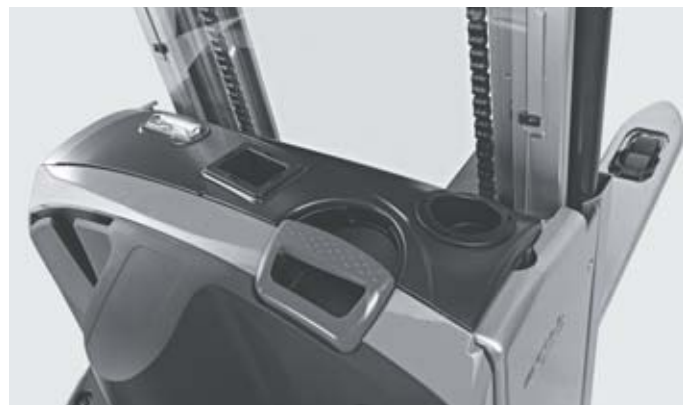
The steel battery cover is not only robust but also provides integrated storage options
