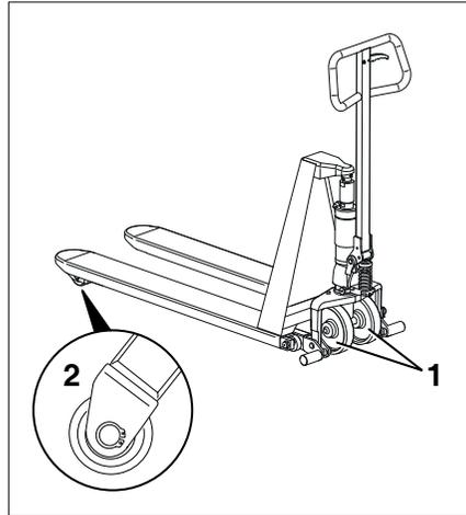
**Checking the mounting of the steering rollers**
