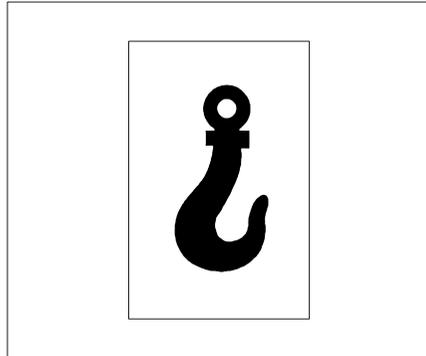
**"Fixing point for the lifting gear" adhesive label**
