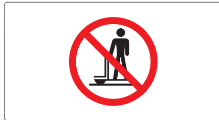
Warning sign on the truck: Lifting of persons with the forks is prohibited
