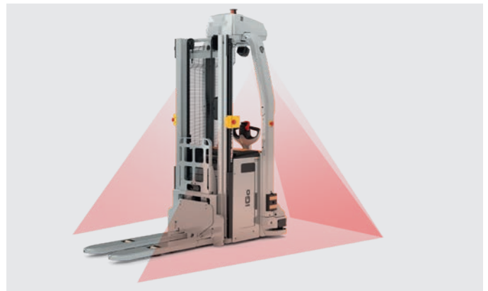
Reliable collision avoidance with additional sensors for detecting obstacles in the truck's environment
