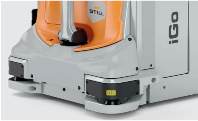
Excellent operator safety thanks to reliable 360-degree safety laser on the truck
