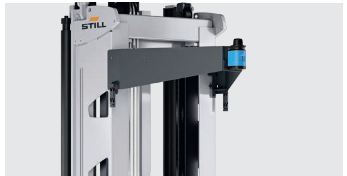
The sensitive navigation laser in the upper area of the truck enables maximum precision, efficiency and safety
