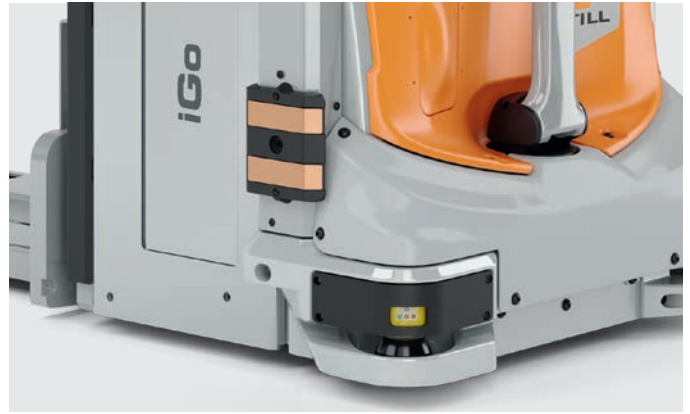
The entire charging process of the EXV iGo can be fully automated: Charging contacts for both lithium-ion and lead-acid batteries
