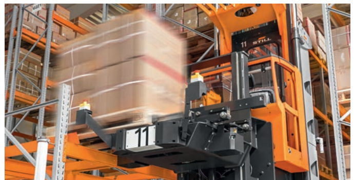
The MX-X iGo is equipped with a telescopic fork for maximum storage density
